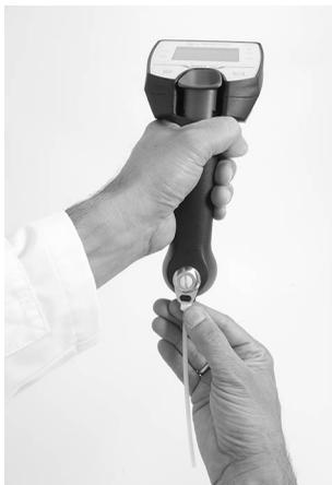
*Fig. 2: Connecting the filling tube*
