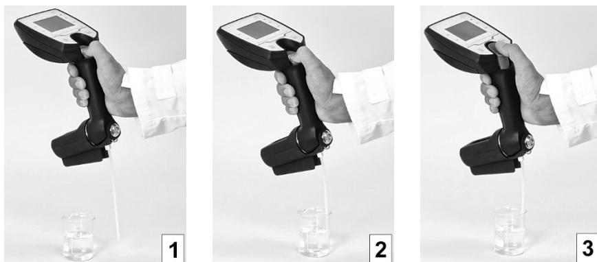
Fig. 7: Filling sample with the filling tube
