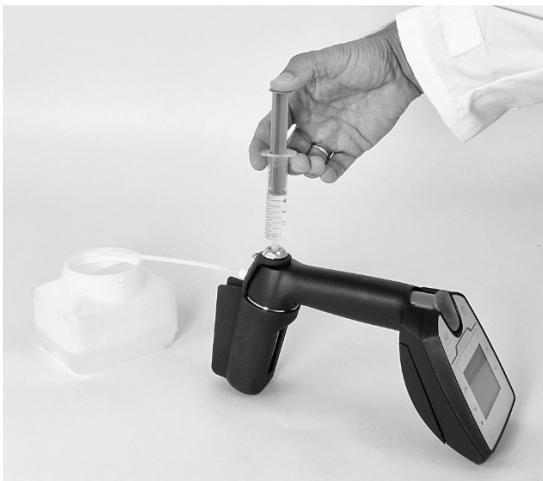
*Fig. 8: Filling sample with a syringe*
