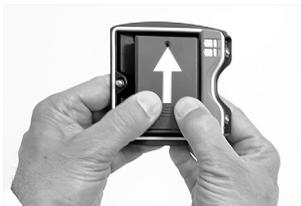
*Fig. 13: Removing the cover of the battery compartment*
